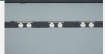
High density Collective Flip chip 20µ Φ Copper pillars
