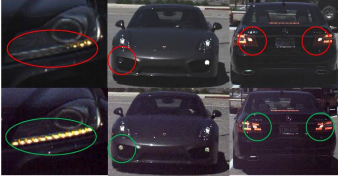
Multi-exposure HDR (top) vs. Pulsed LFM HDR (bottom) image captures of flickering LED Lights
