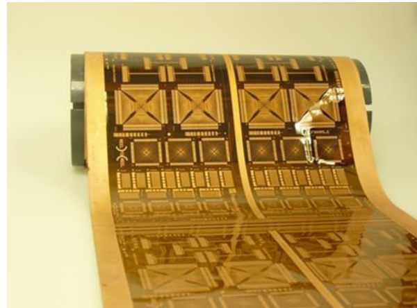
Fig: printed circuit on endless substrate
