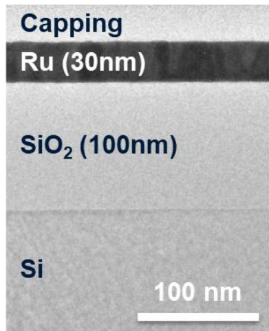
Stack used during this work
