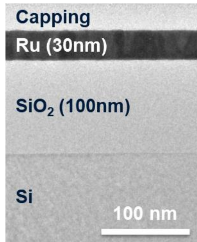
Stack used during this work
