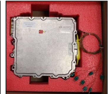
Traction inverter with Power modules in Cu-AIT BOSCH
