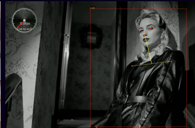
Cascaded pipeline – pose estimation followed by detection in zoomed-in region of interest (ROI) Applied to different use cases (fruit detection, gun detection)
